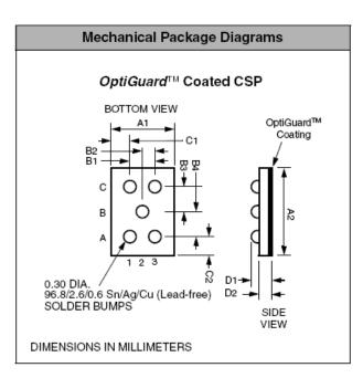
Package Dimensions for CM1204 Chip Scale Package
