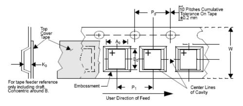
Figure 5. Tape and Reel Mechanical Data
